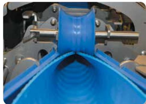
Flat belt is formed into a tube using the guide wheel
