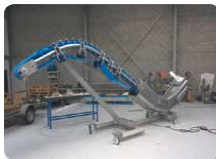
Lowering frame for cleaning
