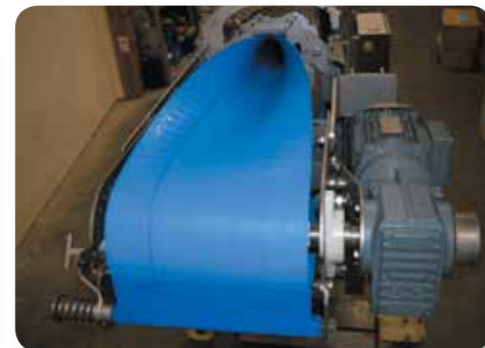
Tube naturally becomes flat at the product exit point
