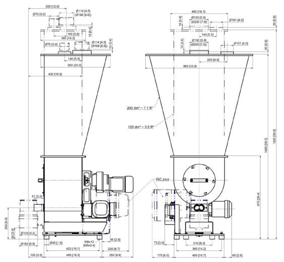
Weight with 100 dm³/3.5 ft³ extension hopper approx. 120 kg (265 lb) Weight with 200 dm³/7.1 ft³ extension hopper approx. 135 kg (298 lb)
