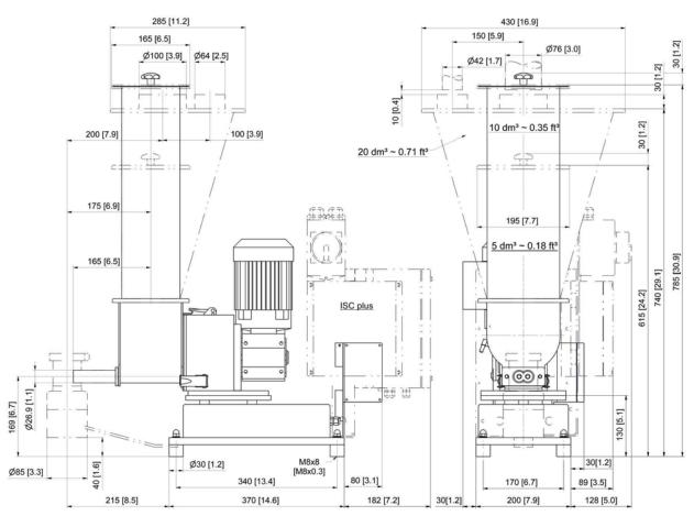
Weight with 5 dm $^3$ /0.18 ft $^3$  extension hopper approx. 29 kg (64 lb) Weight with 10 dm $^3$ /0.35 ft $^3$  extension hopper approx. 31 kg (68 lb) Weight with 20 dm $^3$ /0.71 ft $^3$  extension hopper approx. 35 kg (77 lb)
